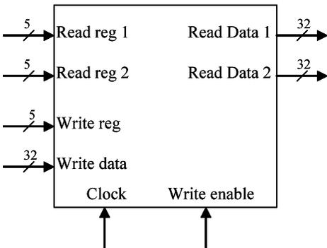
A register file, as discussed in class and the text, is simply a set of registers that can be read from and written to. You will implement a register file with 32 registers of 32 bits each. The register file should be designed using schematic entry in Xilinx; however, components inside the register file such as multiplexors may be created with Xilinx's Coregen tool if desired.
