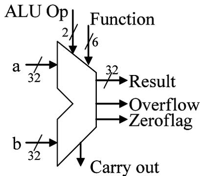
The Arithmetic Logic Unit (ALU) is one of the most fundamental building blocks for computer hardware. You will implement a 32-bit ALU with capability to perform ADD, SUB, AND, OR, SLT, and SRL, along with zero-check and overflow indicators. (Note: SLT must work even in overflow situations.) The ALU may be designed using schematic entry in Xilinx or using HDL. Use any ALU design approach you wish.
