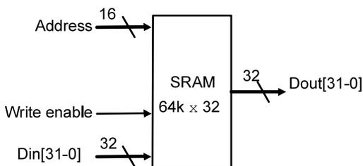
Capability to read and write information to memory is essential to all computer programs. You will implement a 64k x 32 (256kB) Static Random Access Memory (SRAM), i.e. a 16-bit wide address bus and a 32-bit wide data bus. The memory unit may be designed using any approach you wish, including hierarchical schematic design, HDL, or Coregen. The key design criteria is that the memory should be able to be *preloaded* with data using a hex text file (or other similar simple method).
