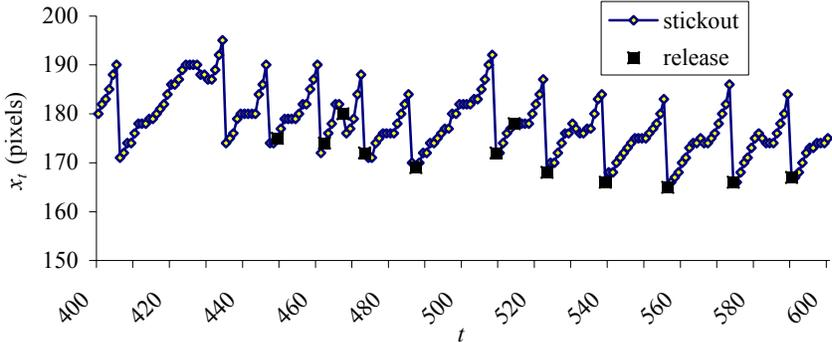
Figure 2 – Welding Stickout and Release Time Series
