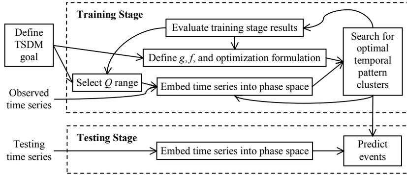
**Figure 3 – Block Diagram of TSDM Method**
